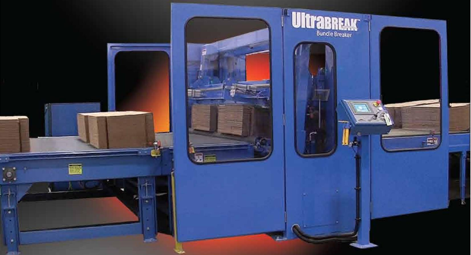
**Faster Cycle Times** are a result of improved controls with optimized position sensing to reduce overall platen travel during the break cycle.
